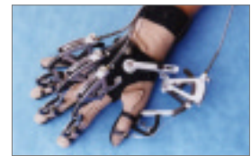
13 Cybergrasp force feedback glove Virtual Technologies, Inc., 1999
